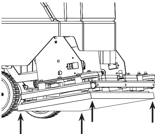
7. With Pad attached securely to Grip Face of EDGE/ORBITZ Deck, the machine is ready to use.
