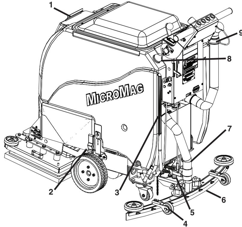
1. **FRONT SOLUTION FILL POINT/LID:** Front fill port for filling Solution Tank
