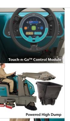
Touch-n-Go<sup>™</sup> control module with 1-Step<sup>™</sup> start button allows operators quick access to all settings without removing hands from the steering wheel.
