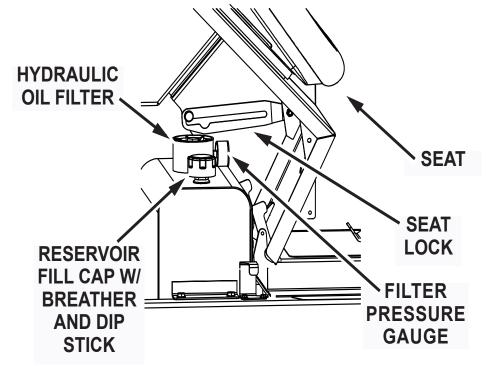
Fig. 2: Hydraulic Fluid Reservoir location
