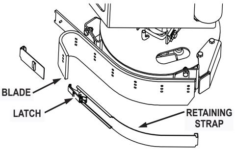
Fig. 3: Retaining Strap & Blade
