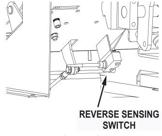
Fig. 3: Reverse Sensing Switch location
