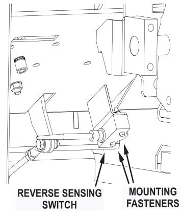
Fig. 1: Reverse Sensing Switch Fasteners
