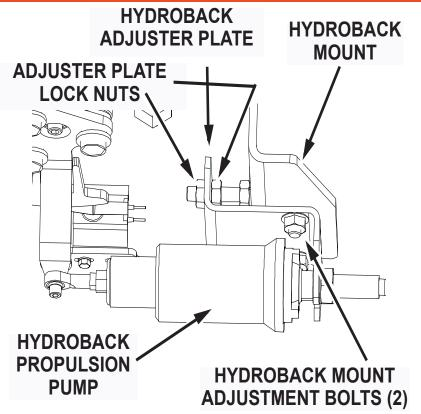
Fig. 1: Hydroback Propulsion Pump
