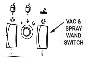
Fig. 2: Vacuum and Spray Wand Switch
