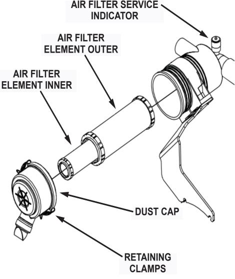
Fig. 1: Air Intake System
