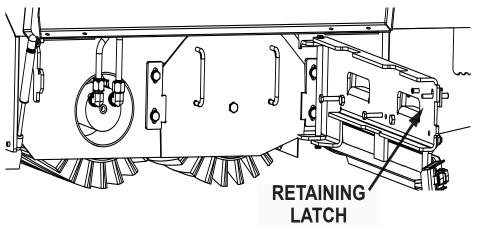
Fig. 1: Retaining Latch location
