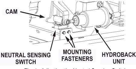
Fig. 1: Adjusting the Neutral Sensing Switch
