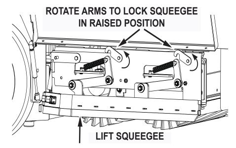
Fig. 1: Shows squeege assembly retaining arms
