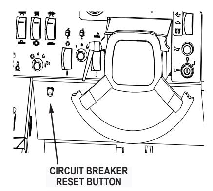
Fig. 1: Circuit Breaker location
