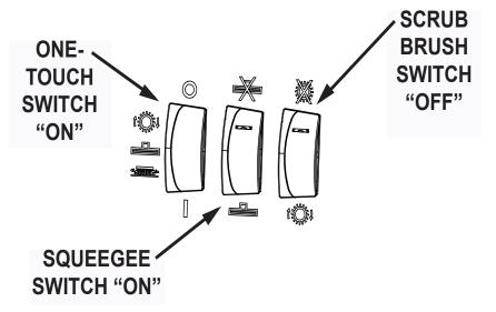
Fig. 1: Control Settings for Water Pick-up Mode
