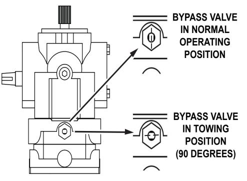
Fig. 2: Bypass Valve locations
