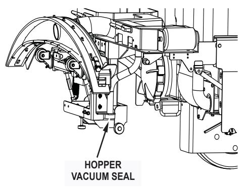
Fig. 3: Hopper Vacuum Seal location
