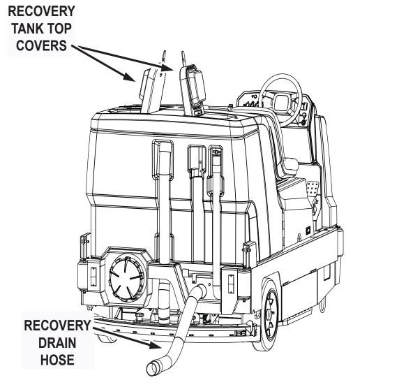
Fig. 1: Draining the Recovery Tank
