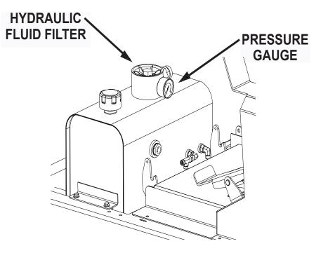
Fig. 2: Hydraulic Filter & Pressure Gauge
