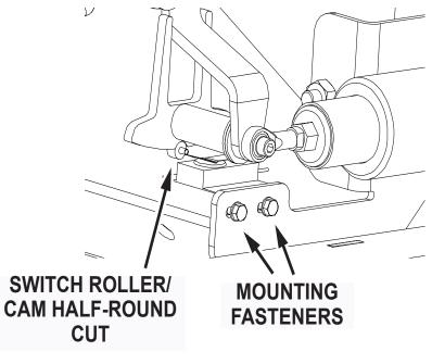
Fig. 2: Roller and Cam Position
