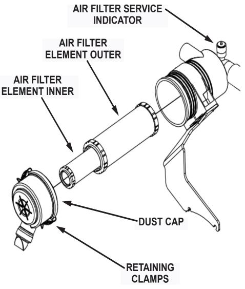
Fig. 1: Air Intake System
