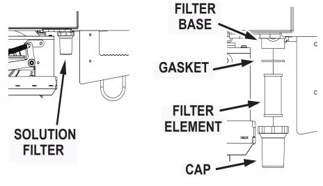
Fig. 2: Water Solution Filter with Exploded view
