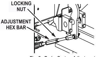
Fig. 2: Brake System Adjustment
