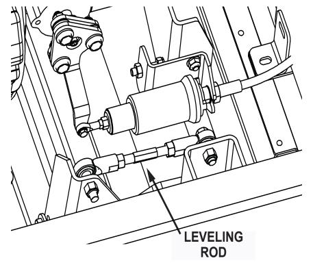
Fig. 4: Leveling Rod location
