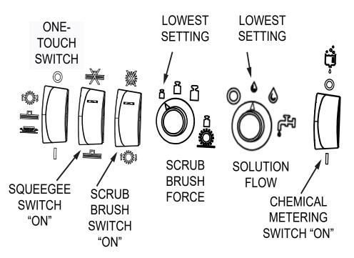
Fig. 2: Control Settings, before "One-Touch" selection
