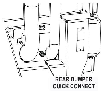
Fig. 1: Spray Wand Quick Disconnect
