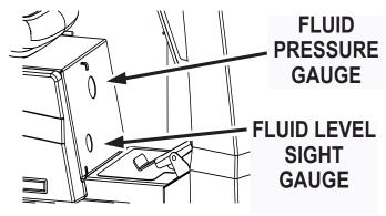
Fig. 3: Hydraulic Fluid Gauges
