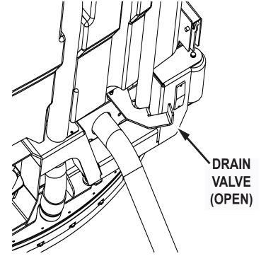
Fig. 2: Drain Valve
