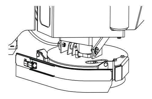
Fig. 1: Replacing the Side Scrub Brush
