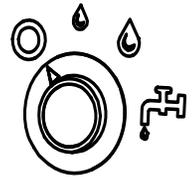
The **Low flow setting** is for normal scrubbing, smooth floors, and light dirt. The flow rate is .88 gal/hr (3,33 L/hr), providing 2.0 hours of scrub time.
