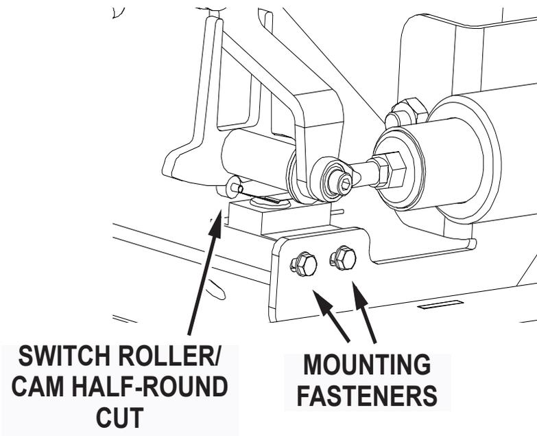
Fig. 2: Roller and Cam Position
