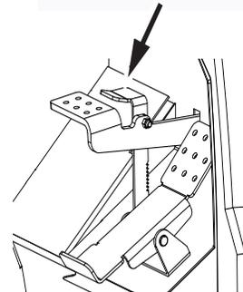
Fig. 2: Set the Praking Brake
