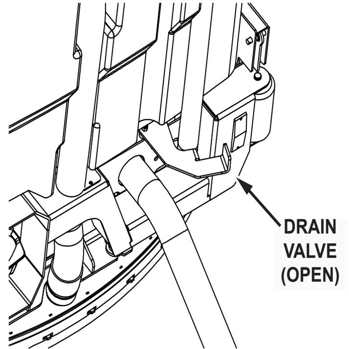
Fig. 2: Drain Valve
