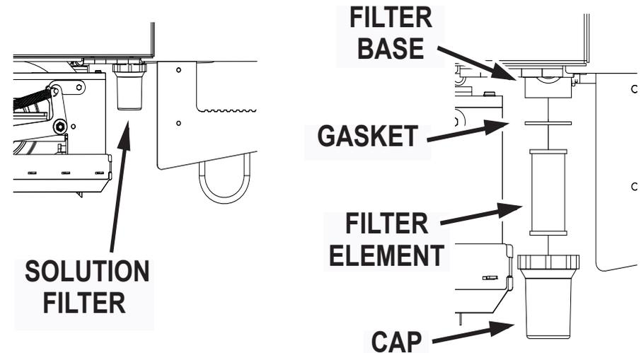
Fig. 2: Water Solution Filter with Exploded view
