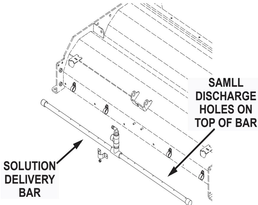
Fig. 1: Solution Delivery Bar shown with holes
