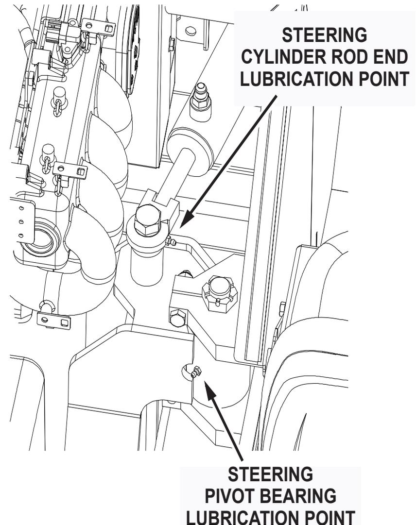
Fig. 1: Lubrication Points
