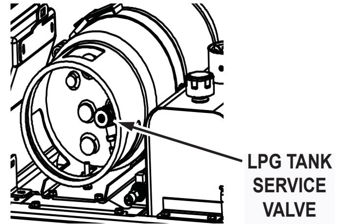
Fig. 1: LPG Tank - Location of Service Valve
