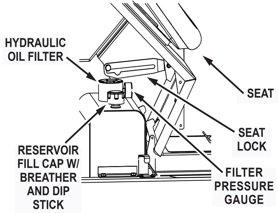
Fig. 2: Hydraulic Fluid Reservoir location
