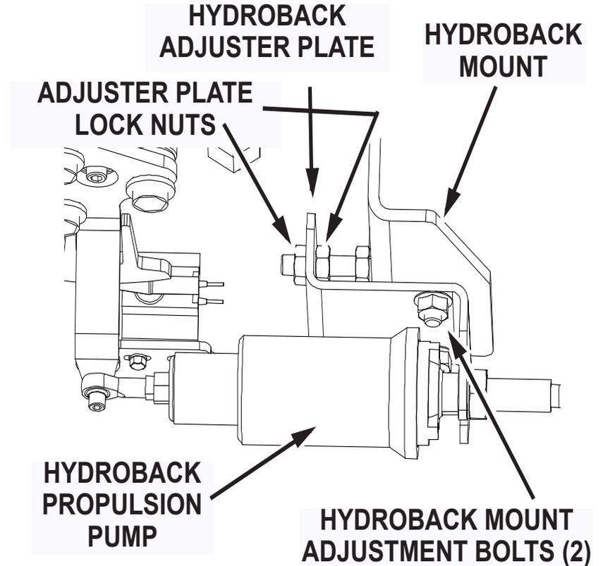
Fig. 1: Hydroback Propulsion Pump
