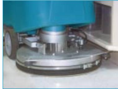
**Low profile scrub deck** cleans tight against edges, in corners, and under obstacles. The unique splash skirt surrounds scrub head to control over spray, conserve water and improve cleaning.
