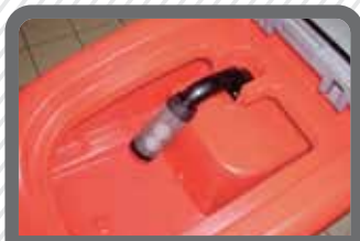
Large Recovery Tank Opening
